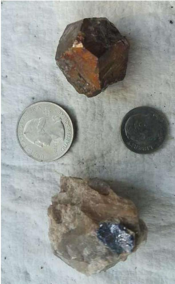
1). Specimens from Benson Mine showing pyritohedron; crystal of molybdenite bottom.
